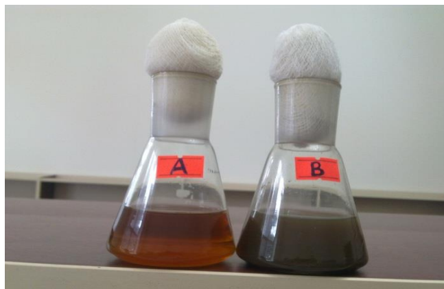
Fig.1. The change of color of reaction medium during formation of silver nanoparticles by strain Saccharomyces sp. BDU-XR1 : a - control variant, b - experimental variant
