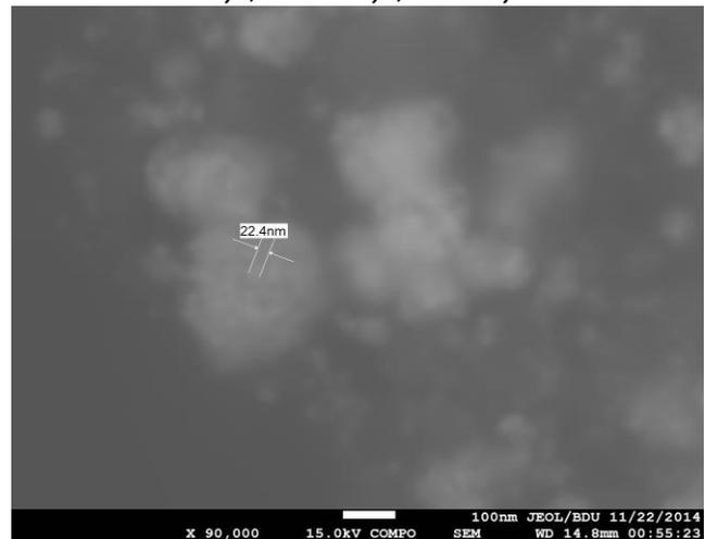
Fig.3. SEM images of silver nanopartiles, synthesized with the biomass of *Actinomyces spp.* NSX-333
