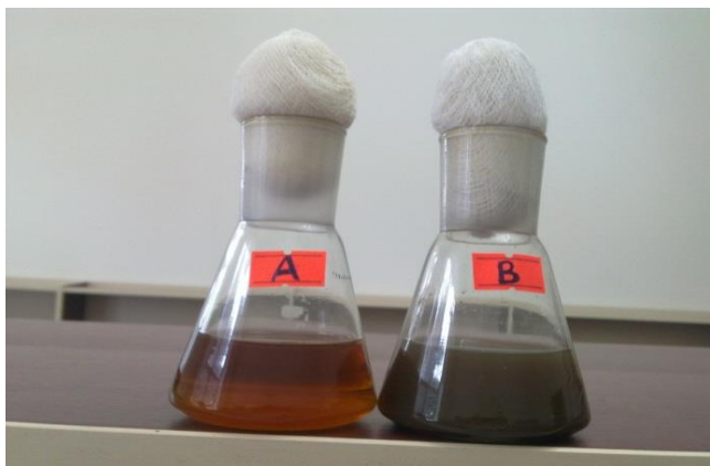
Fig.1. The change of color of reaction medium during formation of silver nanoparticles by strain Saccharomyces sp. BDU-XR1 : a - control variant, b - experimental variant
